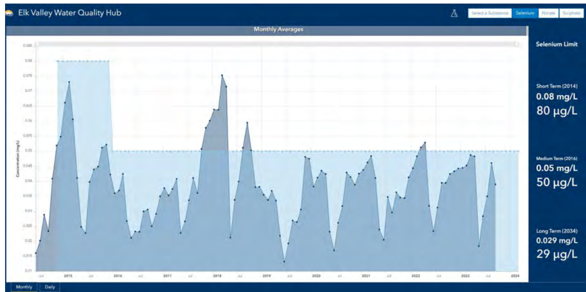
Insert 5-17: Total Selenium Concentrations at Compliance Point Line Creek Mine – Line Creek – 2015 through 2023 (Source: British Columbia Elk Valley Water Quality Hub – Water Quality Data Dashboard)
